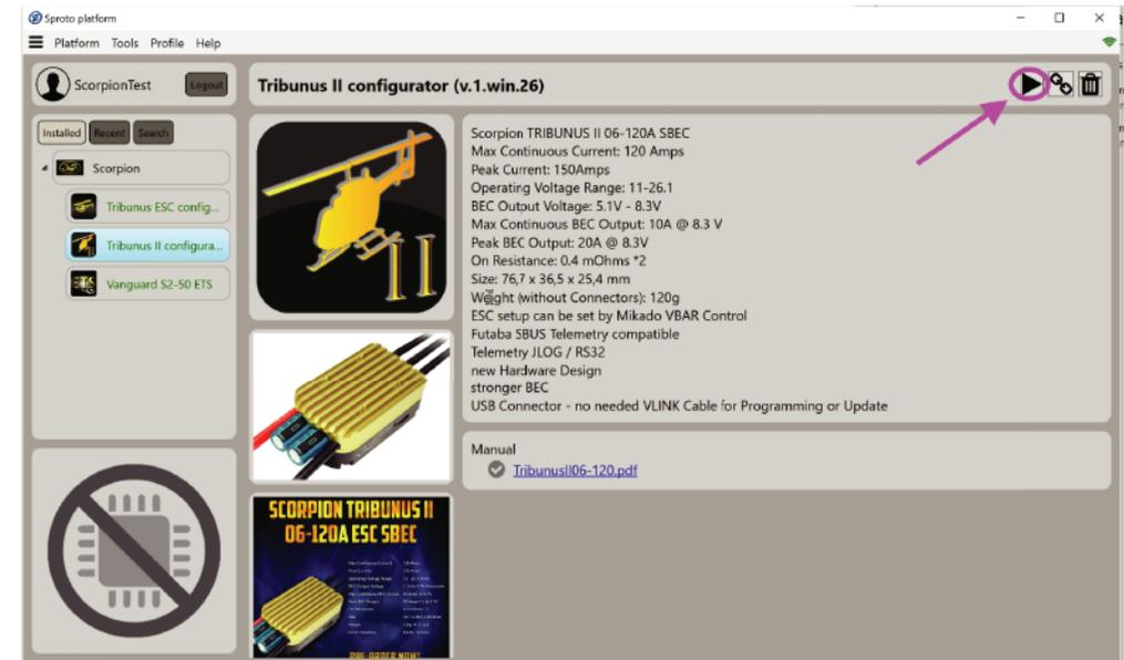
\*\*\*Special Note \*\*\* If your ESC is connecting and then disconnecting constantly then it means you are not using the right configurator. Be sure you are using the proper one.
