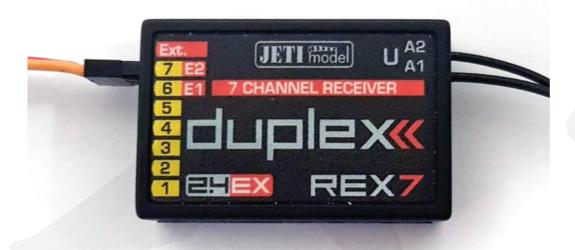
3. Goto Menu -> Model -> Device Explorer -> Rex7 -> Alternative Pin Config and set pin to ExBus (in our example OutPin7/E2 set to ExBus)
