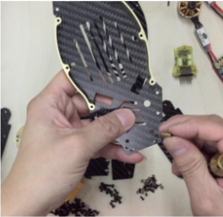
**There are two carbon fibre decks (upper and lower) inside the box. The upper deck is the one pre-assembled with nuts.**
