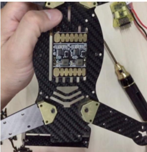
**Solder the motor with the ESC and have a short wiring before assembling on the motor arm.**
