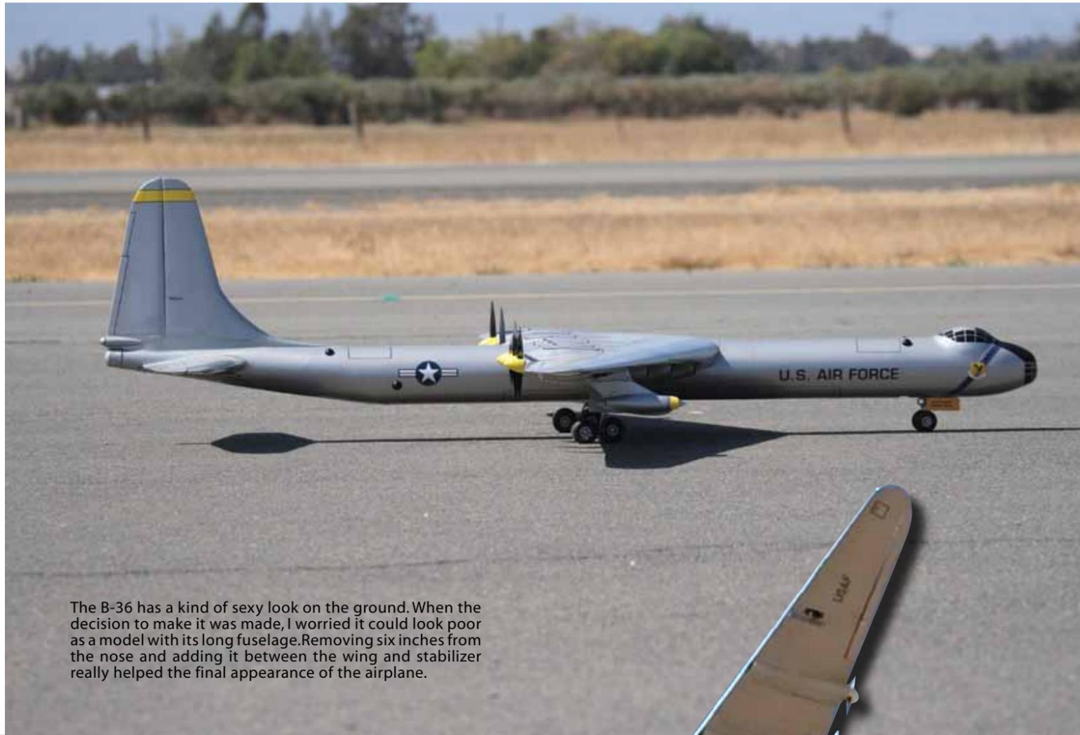
The B-36 has a kind of sexy look on the ground. When the decision to make it was made, I worried it could look poor as a model with its long fuselage. Removing six inches from the nose and adding it between the wing and stabilizer really helped the final appearance of the airplane.
