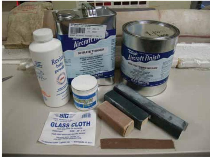
Some of the materials used for this project came from Aircraft Spruce & Specialty, like this nitrate dope and its thinner we used to fill the weave in the fiberglass cloth.
