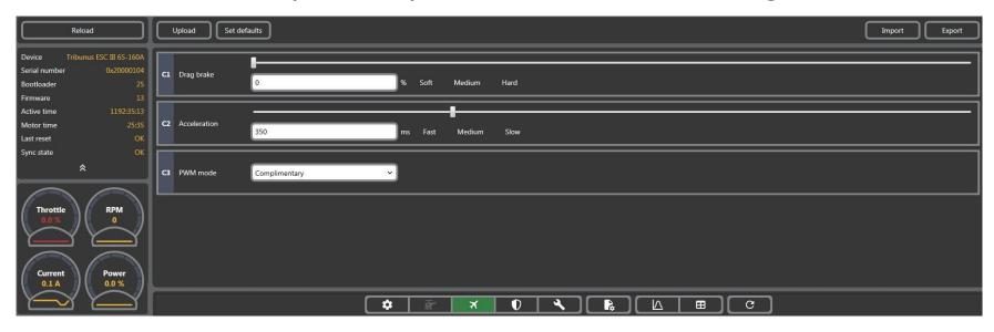
The Tab for this page will change depending on the **Device Mode** which you have selected in Adjustment **A2**. If Airplane mode is selected, then "Plane" tab will appear, same respectively for Airplane with Reverse Mode, and Boat Mode. All 3 mode have the same parameters. You can either click the default presets, Soft/ Medium / Fast, or you may type in a specific value which you prefer.
