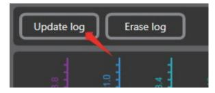
Step 4: Wait for the log to upload to Sproto from the ESC
