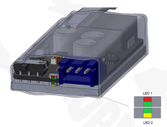
The colors of the LED lights indicate the status/condition of Scorpion Backup Guard II. To operate, the switch of Scorpion Backup Guard II has to be ON.
