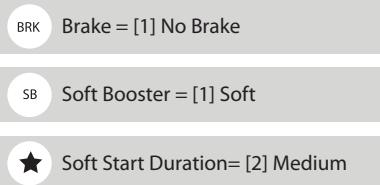
When the throttle stick is in the minimum position and the Heli Mode 1 is enabled, the motor will accelerate slowly until 50% of Power is reached, then the acceleration time will be back to the default setting of MAT (Motor Acceleration Time Delay).
