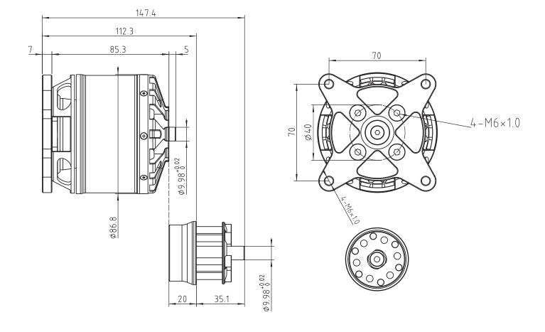
NOTE: The Prop Hub shown is the default selection for this specific size / KV of the A-74 series motor. However, all A-74 Prop Hub options are interchangeable and can be purchased as accessory parts. Motor can as well also be used without Prop Hub, with prop bolting directly to motor face for UAV applications.
